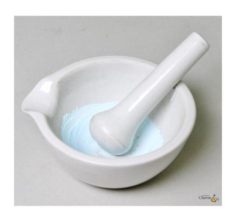
A mortar is used to grind or rub solids.
